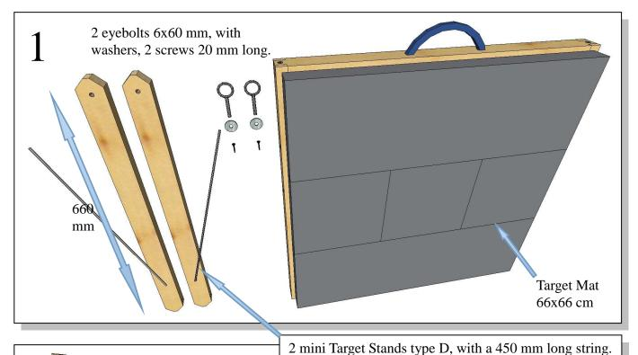
To adjust angle of target, twist the string around the
